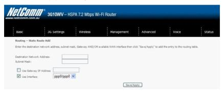
Enter Destination Network Address, Subnet Mask, Gateway IP Address and/or WAN Interface. Then click Save/Apply to add the entry to the routing table.
